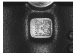
Dot Peening On Scratched Surface
