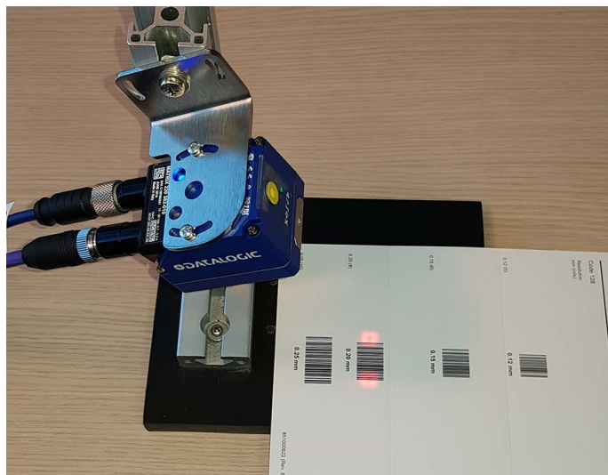
Figure 9 - X-PRESS Interface; Aim/Autofocus Function
