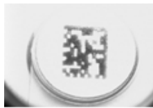
Washed out and Axial Distortion
