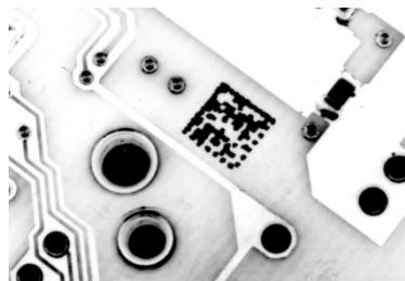
Figure 26 - Data Matrix Code Directly Marked on PCB Surface by Using Laser Etching Technology
