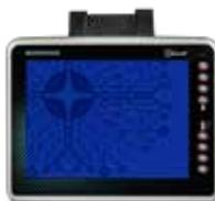
The Rhino II™ vehicle mount computers, available in both 10" and 12" display sizes, sets the standard for ruggedness in the warehouse. Rhino II offers a choice of WEC7, WES 7, Windows 10 IoT Enterprise or Android 7.1 operating systems.
