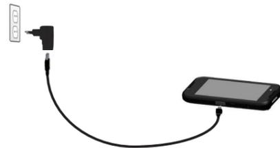
You can also use the USB cable to charge the Memor 10 from any self-powered USB hub or USB port on a computer.
