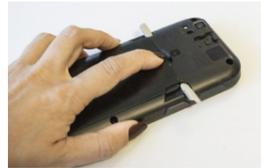
3. Rotate the latches to the lock position to lock the cover:
