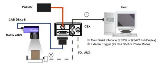
Figure 3 - Matrix 410N in Stand Alone Layout
