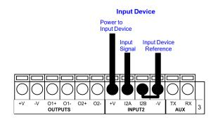
Figure 56 - PNP Input 2 Using Matrix 410N Power
