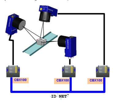
ID-NET interface allows local connection of multiple readers reading different sides of the same target. All readers share a single presence sensor and activate/deactivate simultaneously.
