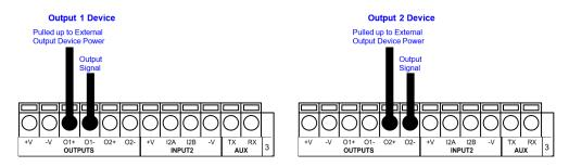
Figure 63 - PNP/Open Emitter Output Using External Power
