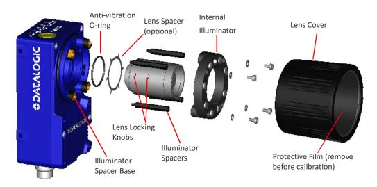
Figure 2 - Assembling Matrix 410N Accessories
