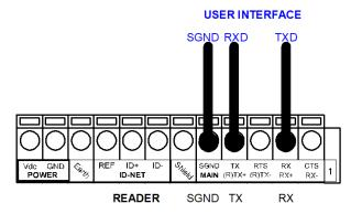
Figure 43 - RS232 Main Interface Connections
