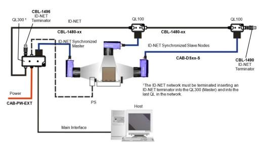
Figure 76 - ID-NET Synchronized Layout Matrix 410N Master with QL300+ Matrix 410N Slaves with QL100
