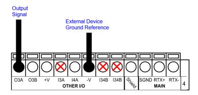
Figure 66 - Output 3 Using External Power
