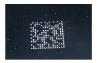
Figure 27 - Directly Marked Dot Matrix Code Characterized by Outstanding Separation
