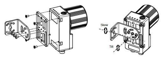
Figure 4 - Positioning with Mounting Bracket (back)
