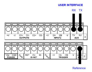
Figure 51 - RS232 Auxiliary Interface Connections
