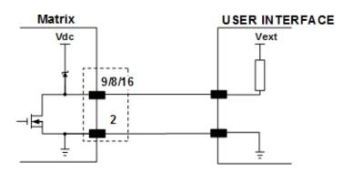
Figure 5 - NPN Output Connection
