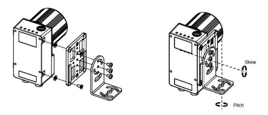
Figure 5 - Positioning with Mounting Bracket (side)
