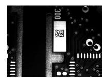
Figure 28 - Dot Matrix Code Directly Marked on PCB Copper Pad by Using Ink-Jet
