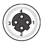
Figure 2 - M12 X-Coded Female Ethernet Network Connector
