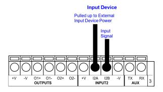
Figure 59 - NPN Input 2 Using External Power
