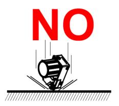
• do not fine tune the positioning by striking the reader or bracket.
