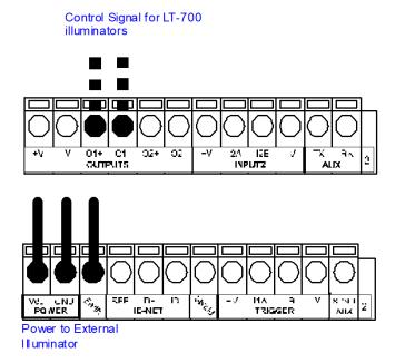
Figure 67 - External Lighting System Connections
