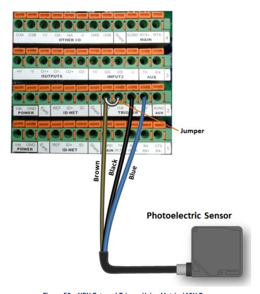
Figure 53 - NPN External Trigger Using Matrix 410N Power
