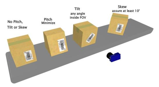
Figure 40 - Pitch, Tilt, and Skew Angles
