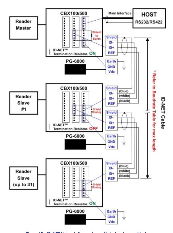
Figure 47 - ID-NET Network Connections with isolated power blocks
