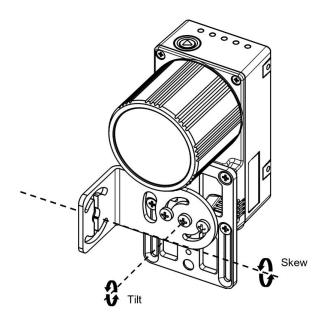
Figure 39 - Positioning with Mounting Bracket (Front)
