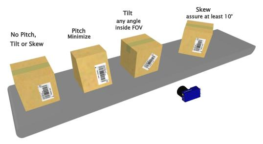
Figure 6 - Pitch, Skew and Tilt Angles
