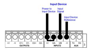
Figure 57 - NPN Input 2 Using Matrix 410N Power
