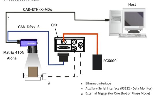
Figure 68 - Ethernet Point-to-Point Layout
