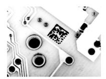
Figure 29 - Data Matrix Code Directly Marked on PCB Surface by Using Laser Etching
