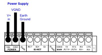
Figure 41 - Power Supply Connections
