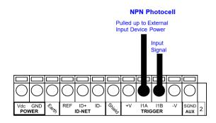
Figure 55 - NPN External Trigger Using External Power
