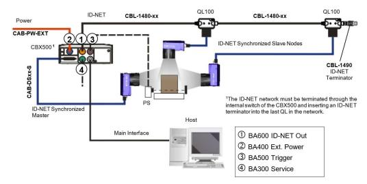
Figure 75 - ID-NET Synchronized Layout Matrix 410N Master with CBX500 + Matrix 410N Slaves with QL100
