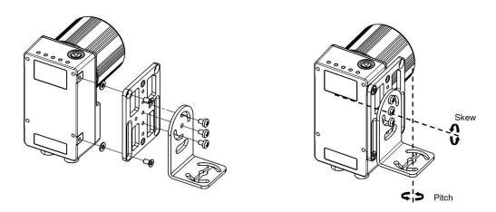
Figure 38 - Positioning with Mounting Bracket (Side)
