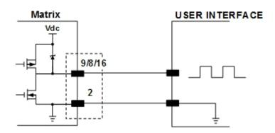
Figure 6 - Push-Pull Output Connection
