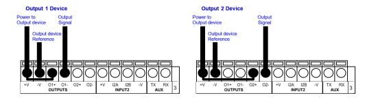
Figure 61 - PNP/Open Emitter Output Using Matrix 410N Power
