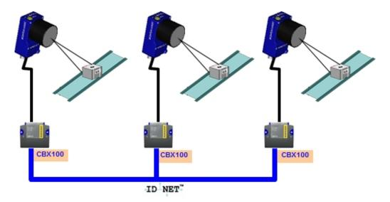
ID-NET interface allows connection of readers reading objects placed on independent conveyors. All readers are typically located far away from each other and they can have different operating modes from each other.
