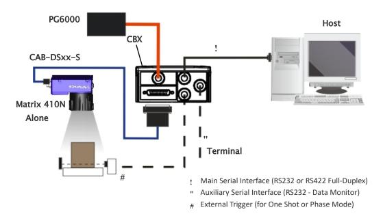
Figure 70 - Serial Interface Point-to-Point Layout
