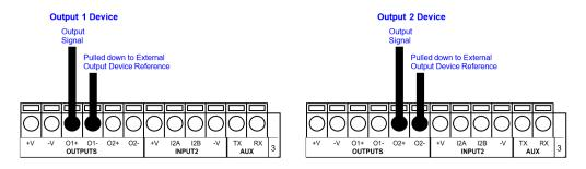
Figure 64 - NPN/Open Collector Output Using External Power
