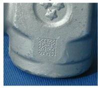
Figure 25 - Dot Matrix Code Directly Marked on Metal Surface by Using Dot Peening
