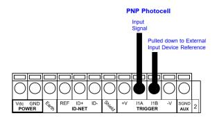
Figure 54 - PNP External Trigger Using External Power
