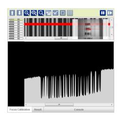
8. Click the Acquire PPI button to automatically set Image Density so that Matrix 410N will function correctly and to the fullest extent of its capabilities. This procedure is necessary for first time installations, or if the lens type or focal distance is changed.
