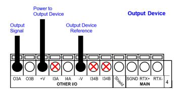
Figure 65 - Output 3 Using Matrix 410N Power
