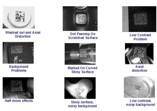
Figure 85 - Problematic Direct Part Marking Examples
