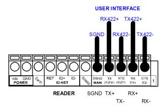
Figure 44 - RS422 Full Duplex Connections
