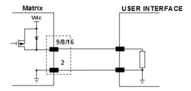
Figure 4 - PNP Output Connection
