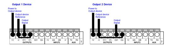
Figure 62 - NPN/Open Collector Output Using Matrix 410N Power
