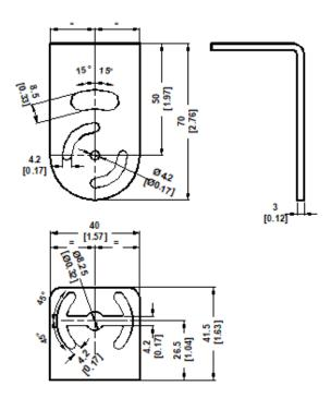
Figure 36 - Mounting Bracket Overall Dimensions
