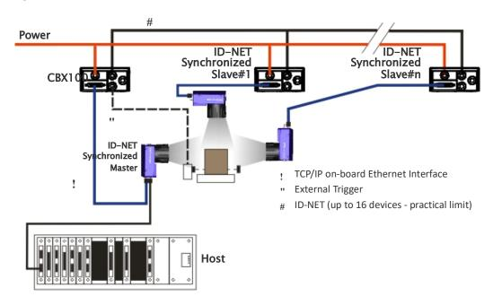
Figure 77 - ID-NET Synchronized Layout with Master on-board TCP/IP Ethernet
