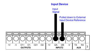
Figure 58 - PNP Input 2 Using External Power
