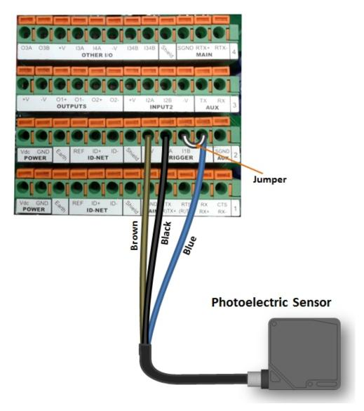
Figure 52 - PNP External Trigger Using Matrix 410N Power
