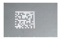
Figure 26 - Dot Peening Marking on Metal Surface with Multi-dot per Code Element
