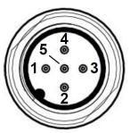
Figure 3 - M12 X-Coded Female Ethernet Network Connector
