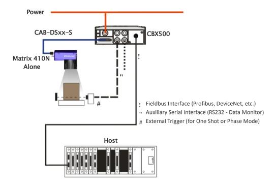
Figure 71 - Fieldbus Interface Point-to-Point Layout
