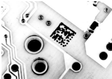
Figure 27 - Data Matrix Code Directly Marked on PCB Surface by Using Laser Etching Technology
