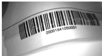
Figure 22 - Barcode Printed on Curved Surface Readable by Matrix 300N in spite of Image Optical Distortion
