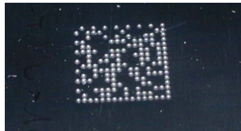
Figure 25 - Directly Marked Dot Matrix Code Characterized by Outstanding Separation Distance between Adjacent Code Elements
