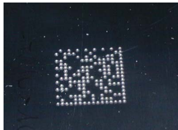
Figure 22 - Directly Marked Dot Matrix Code Characterized by Outstanding Separation Distance between Adjacent Code Elements
