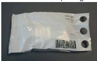
Figure 17 - Unidose Flow-Pack with PDF417 Code
