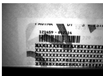
Figure 18 - Overprinted Barcode Readable by Matrix 300N also Through the Envelope Window Film
