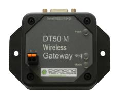
On the serial side the DT50 supports RS232, RS485 and optionally RS422 for use in multidrop environments and where longer cable runs are needed to serial devices. Serial communications support speeds up to 115.2K baud on Bluetooth LE models and 1.25M baud on Classic Bluetooth models, for fast data transmission over a wide range of applications.
