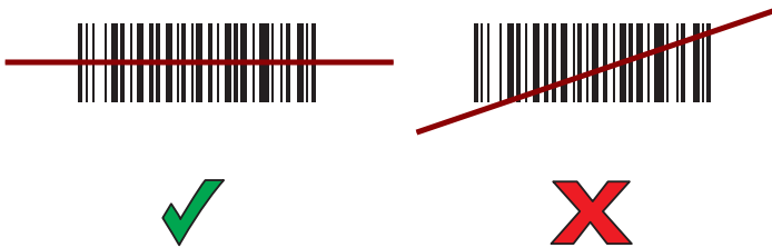
Figure 40 Laser Scanner Aiming Pattern
