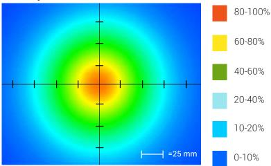
Optical measurement taken using SL073-WHIIC @ 300 mm
