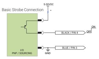
\*External resistors may not be needed Check documentation on I/O for recommendations and voltage limits
