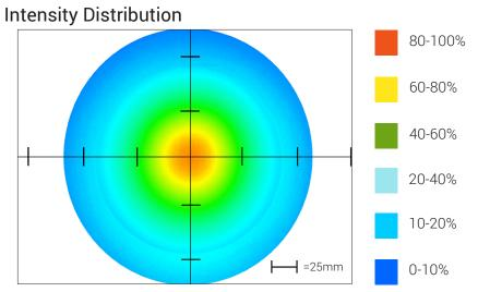
Optical measurement taken using RL3536-625I3 @ 75mm
