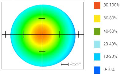
Optical measurement taken using RL2316-625100LI3 @ 100 mm
