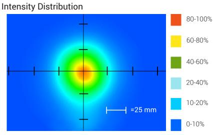
Optical measurement taken using RL2115-WHII3 @ 9.5 mm
