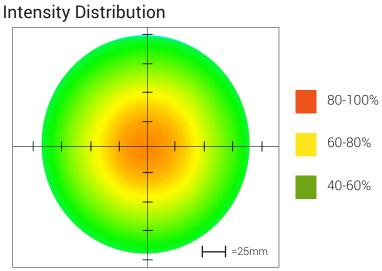
Optical measurement taken using RL127-WHIIC @ 200 mm
