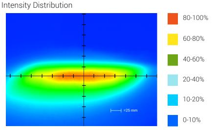
Optical measurement taken using LL15812-62524 @ 75 mm
