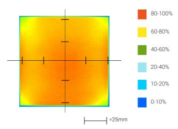
Optical measurement taken using CX0404-WHIIC
