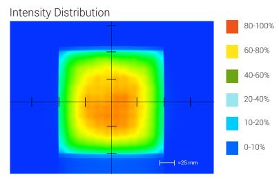
Optical measurement taken using BL128-WHIIC
