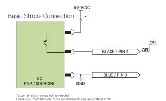
Analog dimming works in both strobe and continuous
