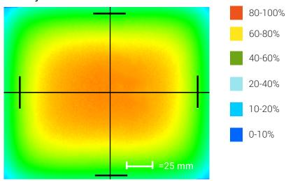
Optical measurement taken using BL-S050075-WHI
