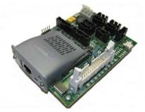
DT7000 Embedded Gateway, Digital and Analog I/O, Serial Communications, Support for most major industrial communication protocols, embedded user C programming environment, IoT platform.
