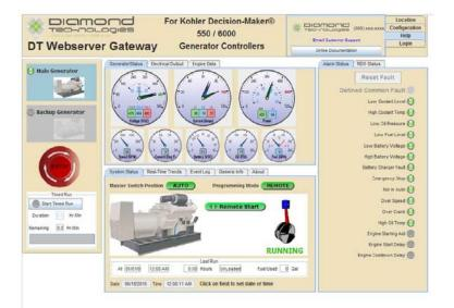
Diesel Generators provide 24/7 backup power to critical applications such as hospitals, data centers, and financial institutions. **Diamond Technologies** Webservers provide 24/7 monitoring, alarming, and remote testing of these critical infrastructure systems.
