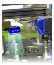
MA.R.V.I.S. (MArk Read Verify Integrated Solution) is the new Datalogic solution that ensure quality of laser marked 2D codes.
