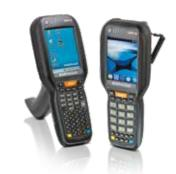
The Falcon™ X4 mobile computer features a high performance multicore 1 GHz architecture that offers blazing speed when running Windows Embedded Compact OS and allows easy upgradeability to the Android™ OS.
