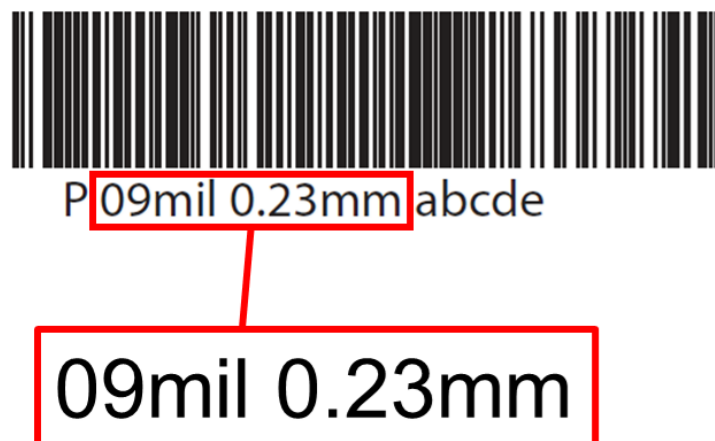
Figure 119: Picket Fence/Step Ladder Res Test Chart barcode example
