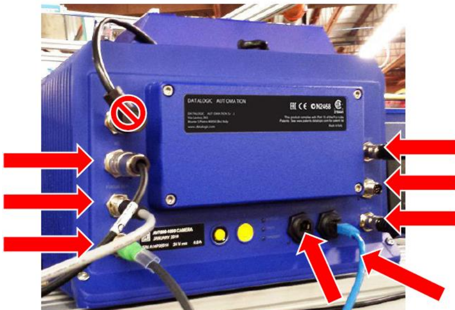
Figure 126: Remove the cables
