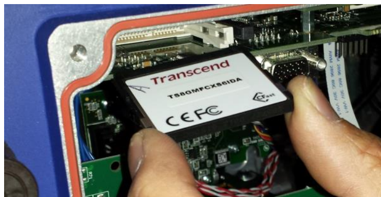
Figure 125: Removing the memory card
