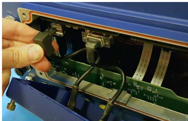
Figure 92: Connecting USB Cable
