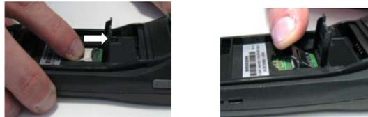
5. Insert the microSD card with the written part upward:
