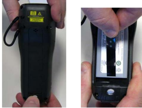
3. Open the microSD card slot by lifting up the locking plate:
