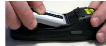
3. Reinsert the cover. First insert first the upper side and then press the latch release button and pull the latch down to insert the bottom. Push the knurled section of the latch upwards to close the cover:
