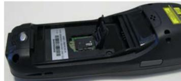
6. Lock the card into place by pushing the cardholder down and then shifting it downwards; push the locking plate down:
