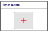
The field of view indicated by the aiming system will be smaller when the reader is closer to the bar code and larger when it is farther from the code. Symbologies with smaller bars or elements (mil size) should be read closer to the unit. Symbologies with larger bars or elements (mil size) should be read farther from the unit. If the entire bar code is within the aiming field, you will get a good read. Successful reading is signaled by an audible tone plus a good-read green spot LED indicator.
