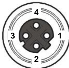
Figure 86 - M12 D-Coded 4-pin Female PROFINET-IO Network Connector
