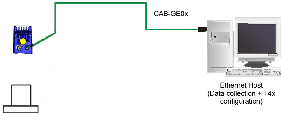
Figure 41 - Standalone Layout to Ethernet Host (Point-to-Point)
