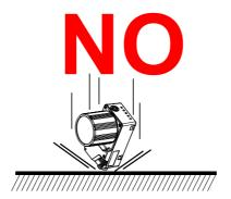
• do not fine tune the positioning by striking the reader or bracket.
