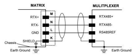
Figure 85 - RS485 Half-duplex Connections
