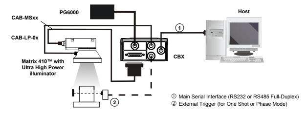
Figure 3 – Matrix 410 655-0x0 Models in Stand Alone Layout
