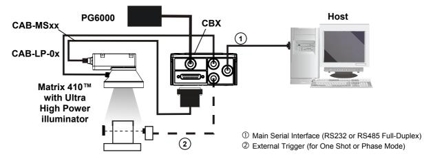
Figure 106 - Serial Interface Point-to-Point Layout
