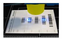
4. Exit the Focus function by pressing the X-PRESS™ push button once. The Blue Diamonds™ turn off.
