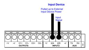
Figure 71 - NPN Input 2 Using External Power
