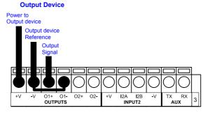
Figure 73 - Open Collector Output Using MATRIX 410™ Power
