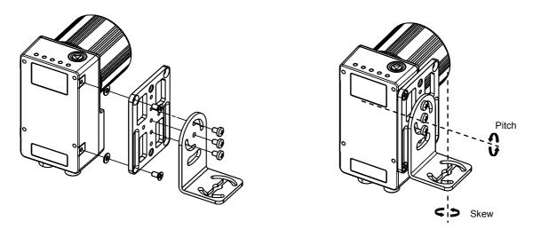
Figure 5 - Positioning with Mounting Bracket (Side)
