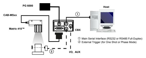
Figure 2 - Matrix 410™ in Stand Alone Layout
