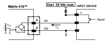
Figure 100 - Input PNP Using External Power
