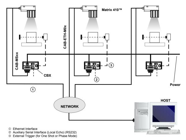
Figure 122 - Ethernet Network Layout
