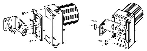
Figure 46 –Positioning with Mounting Bracket (Back)
