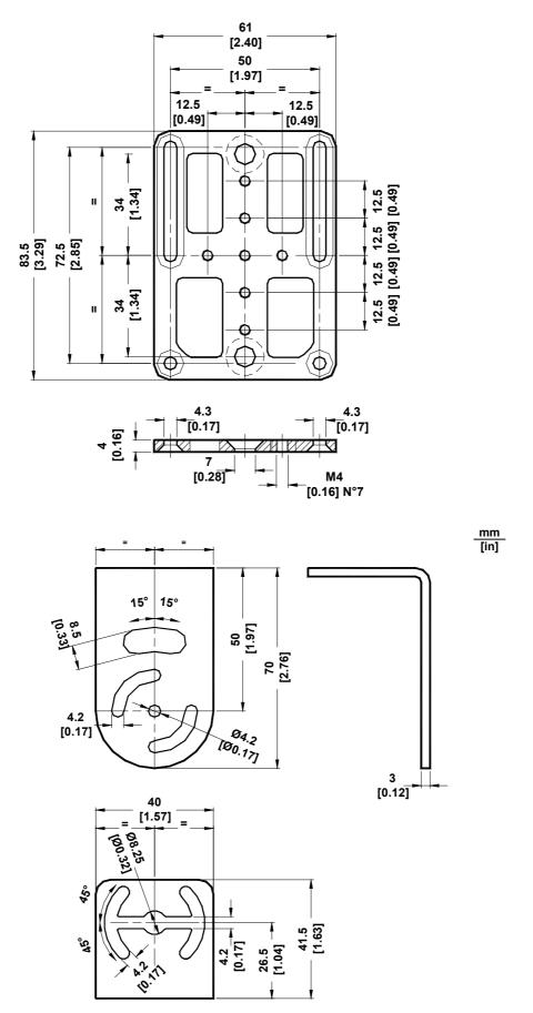
Figure 45 - Mounting Bracket Overall Dimensions
