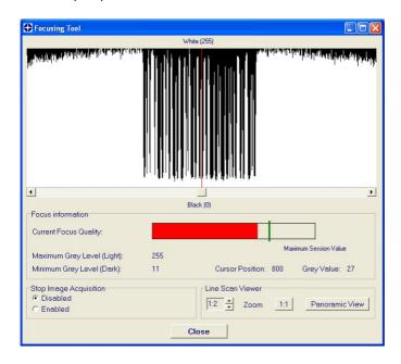
Rotate the Focusing ring in the opposite direction. The Current Focus Quality Bar (green) increases towards the vertical optimal focus line (green) until the optimal focus is reached; the Current Focus Quality Bar touches the vertical optimal focus line (indicating the best focus).
