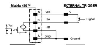
Figure 94 – External Trigger PNP Using Matrix 410™ Power
