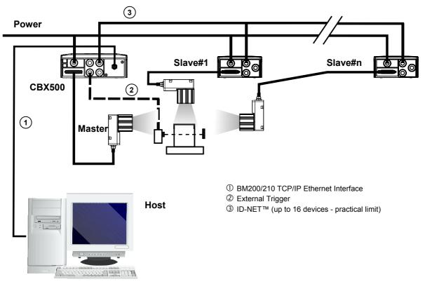
Figure 114 – ID-NET™ M/S Synchronized Layout with BM200/210 TCP/IP Ethernet Interface to Host
