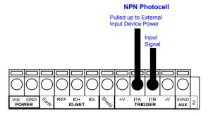
Figure 69 - NPN External Trigger Using External Power
