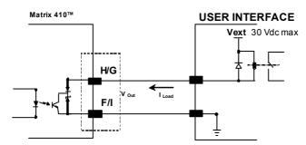
Figure 103 - Open Collector Output Connection
