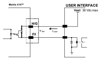
Figure 102 - Open Emitter Output Connection
