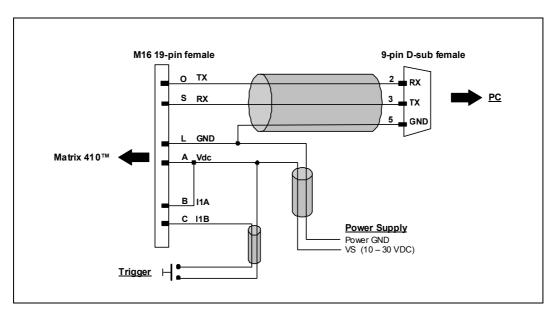
Figure 104- Test Cable for Matrix 410™
