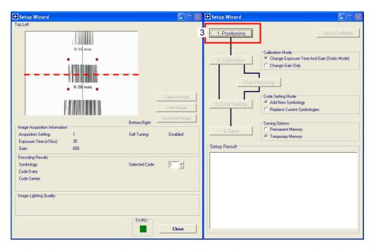
4. Select a Calibration Mode choice and press the "Calibrate" button. The reader flashes once acquiring the image and auto determines the best exposure and gain settings. If the code symbology is enabled by default, the code will also be decoded.
