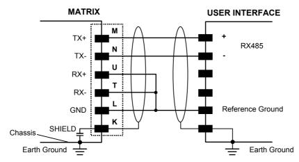
Figure 84 - RS485 Full-duplex Connections using Only TX Signals
