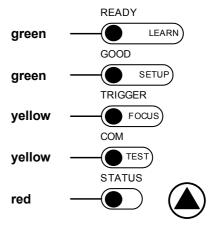
Figure 14 – X-PRESS™ Interface: Learn Function
