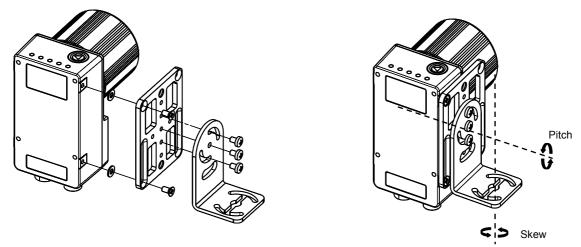
Figure 47 –Positioning with Mounting Bracket (Side)
