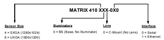
In addition to the basic models, Matrix 410 655-0x0 is available with a pre-mounted 35 mm lens and a pre-mounted Ultra High Power internal illuminator (which is not sold as a separate accessory).
