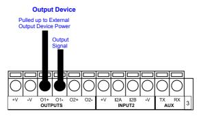
Figure 74 - Output Open Emitter Using External Power
