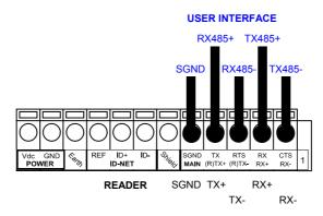
Figure 56 - RS485 Full-duplex Connections
