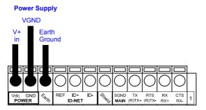
Figure 52 - Power Supply Connections
