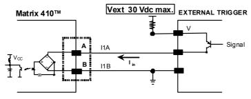
Figure 96 - External Trigger PNP Using External Power
