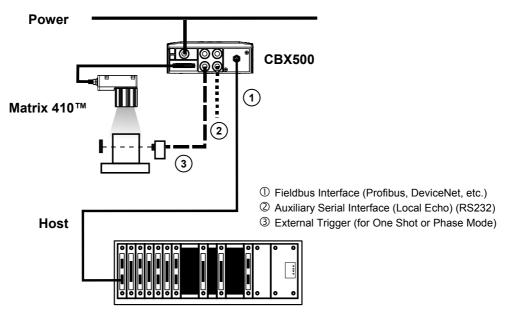
Figure 108 - Fieldbus Interface Point-to-Point Layout
