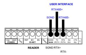
Figure 58 - RS485 Half-duplex Connections
