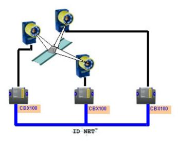
ID-NET™ interface allows local connection of multiple readers reading different sides of the same target. All readers share a single presence sensor and activate/deactivate simultaneously.
