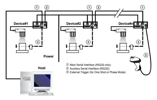
Figure 109 - Pass-Through Layout
