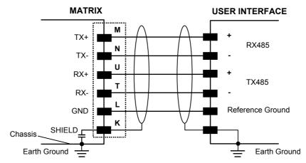
Figure 83 - RS485 Full-duplex Connections
