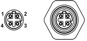
Figure 78 - M12 D-Coded Female Ethernet Network Connector
