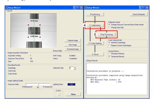
5. Press the "Fine Focusing" button to activate the Fine Focusing Tool.
