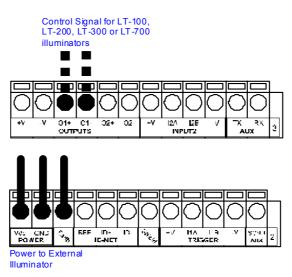
Figure 76 - External Lighting System Connections
