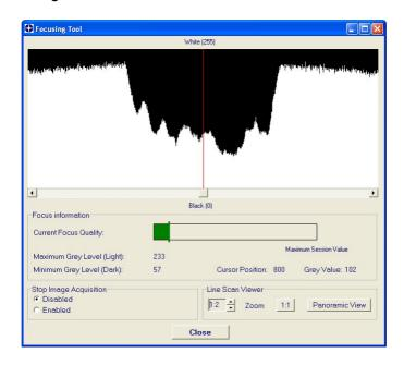
Rotate the Focusing ring on the lens. The Current Focus Quality Bar (green) together with the vertical optimal focus line (green) **increase together** until the optimal focus is reached; the vertical optimal focus line stops.
