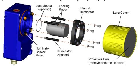
Figure 1 - Assembling Matrix 410™ Accessories
