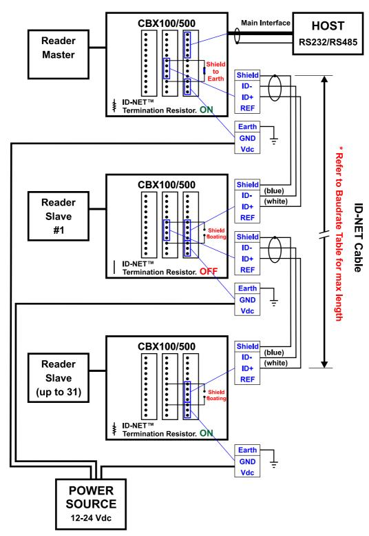
Figure 63 – ID-NET™ Network Connections with Common Power Star Network
