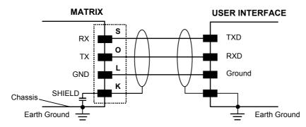
Figure 91 - RS232 Auxiliary Interface Connections Using 19-pin Connector
