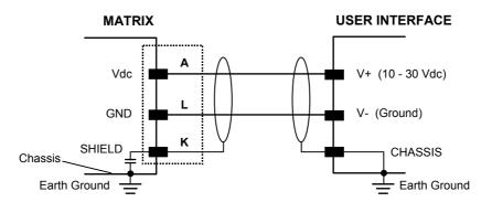
Figure 79 - Power Supply Connection
