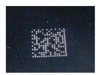
Figure 28 - Directly Marked Dot Matrix Code Characterized by Outstanding Separation Distance between Adjacent Code Elements
