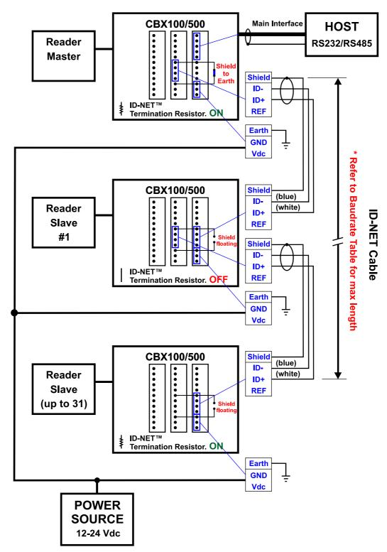
Figure 62 - ID-NET™ Network Connections with Common Power Branch Network
