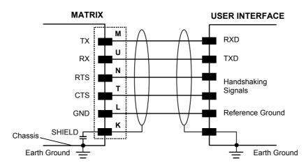
Figure 81 - RS232 Main Interface Connections
