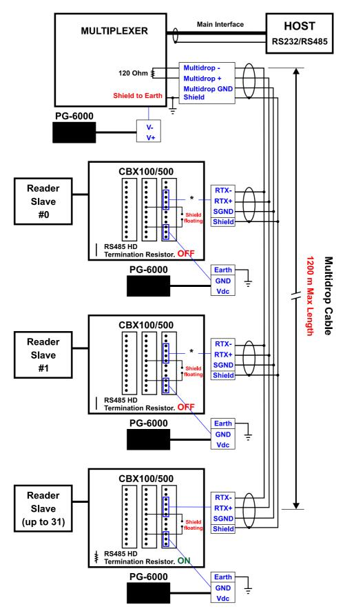
Figure 59 - Matrix 410™ Multidrop Connection to a Multiplexer
