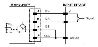
Figure 98 - Input PNP Using Matrix 410™ Power
