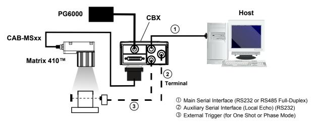
Figure 105 - Serial Interface Point-to-Point Layout
