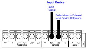
Figure 70 - PNP Input 2 Using External Power
