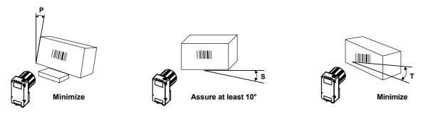
Figure 6 - Pitch, Skew and Tilt Angles
