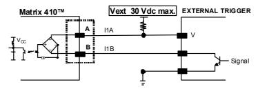
Figure 97 - External Trigger NPN Using External Power
