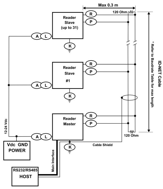
Figure 89 - ID-NET™ Network Connections with Common Power Branch Network
