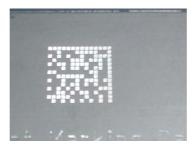
Figure 27 - Dot Peening Marking on Metal Surface with Multi-dot per Code Element
