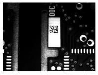
Figure 30 - Dot Matrix Code Directly Marked on PCB Copper Pad by Using Ink-Jet Technology
