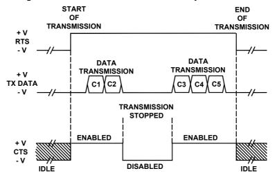
Figure 55 - RS232 Control Signals
