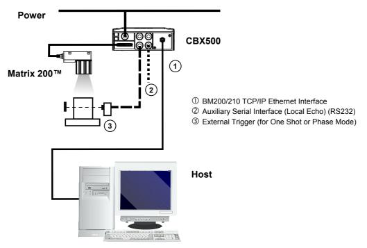
Figure 107 – BM200/210 TCP/IP Ethernet Interface Point-to-Point Layout
