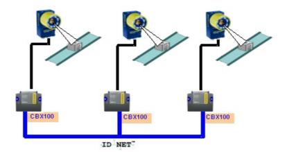
ID-NET™ interface allows connection of readers reading objects placed on independent conveyors. All readers are typically located far away from each other and they use a dedicated presence sensor.
