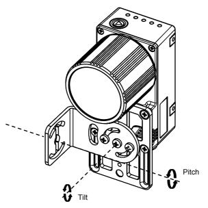
Figure 48 –Positioning with Mounting Bracket (Front)
