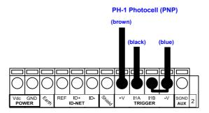
Figure 66 – PH-1 External Trigger Using MATRIX 410™ Power
