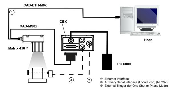
Figure 121 - Ethernet Point-to-Point Layout
