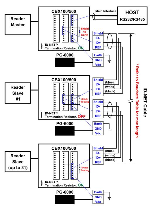
Figure 61 – ID-NET™ Network Connections with isolated power blocks
