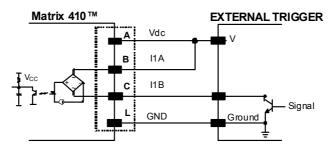
Figure 95 - External Trigger NPN Using Matrix 410™ Power
