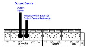
Figure 75 - Output Open Collector Using External Power
