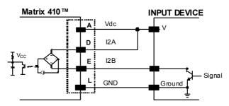
Figure 99 - Input NPN Using Matrix 410™ Power
