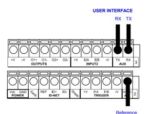
Figure 65 - RS232 Auxiliary Interface Connections
