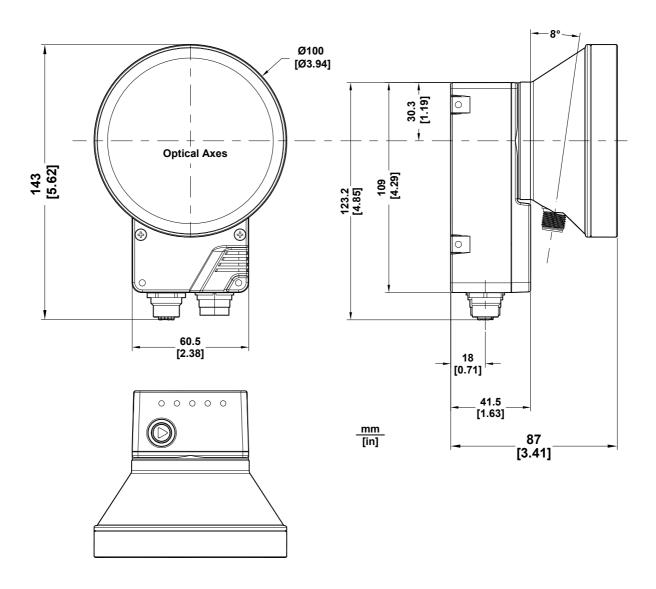
Figure 44 - Matrix 410 655-0x0 Model Overall Dimensions
