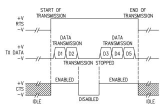
Figure 82 - RS232 Control Signals
