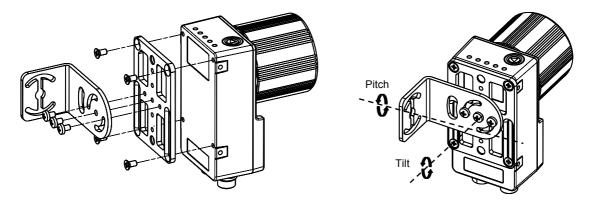
Figure 4 -Positioning with Mounting Bracket (Back)
