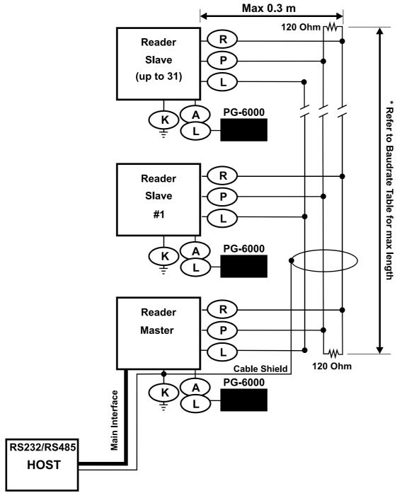
Figure 88 – ID-NET™ Network Connections with isolated power blocks
