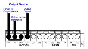
Figure 72 - Open Emitter Output Using MATRIX 410™ Power
