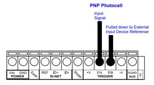
Figure 68 - PNP External Trigger Using External Power
