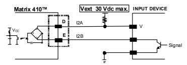
Figure 101 - Input NPN Using External Power
