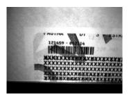
Figure 16 - Overprinted Barcode Readable by Matrix 300™ also Through the Envelope Window Film
