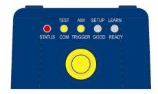
Figure 4 – X-PRESS™ Interface: Aim/Autofocus Function
