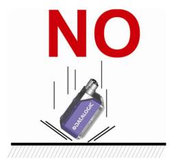
do not fine tune the positioning by striking the reader or bracket.
