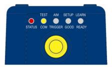
Figure 10 - X-PRESS™ Interface: Test Function
