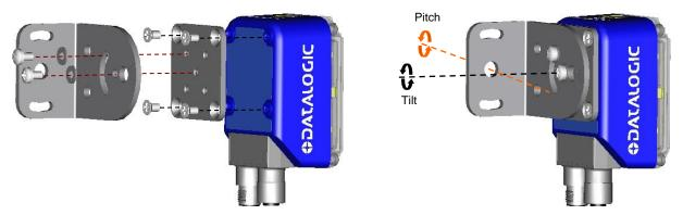
Figure 2 -Positioning with Mounting Bracket
