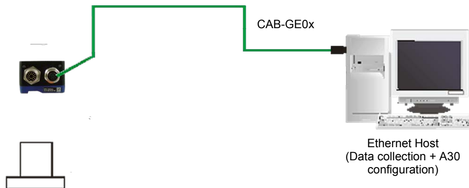
Figure 44 - Standalone Layout to Ethernet Host (Point-to-Point)
