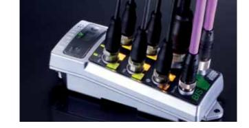
Typical application combining multiple read/write heads with local I/O include tracking and traceability of material or parts in assembly line WIP applications and inter-logistics in automotive, industrial equipment, electronics, medical and packaging.
