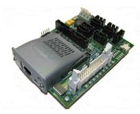
**DT7000** Embedded Gateway, Digital and Analog I/O, Serial Communications, Support for most major industrial communication protocols, embedded user C programming environment, IoT platform.
