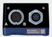
**A** - M16 Male 19 poles (I/O & Power) **B** - M12 Female 8 poles A-Coded (Gigabit Ethernet)
