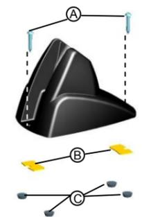
The stand can be mounted by using self-tapping screws, double sided adhesive strips or rubber feet:
