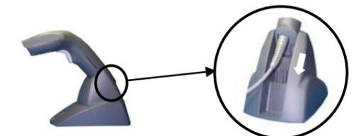
Pair the reader to the stand, taking care to insert the handle into the stand clip (see figure above). Correct insertion will be signaled by a beep; then, the reader will be ready to read barcodes.
