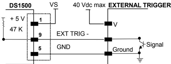
Figure 14 - External Trigger Input Command using External Power
