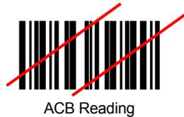
ACB reads two fragments of a label containing a start or a stop character and a number of digits, and puts them together to build the complete label.
