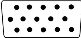
Figure 5 - 15-pin D-sub High-Density Male Connector
