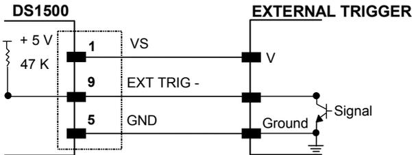
Figure 13 - External Trigger Input Command using Scanner Power
