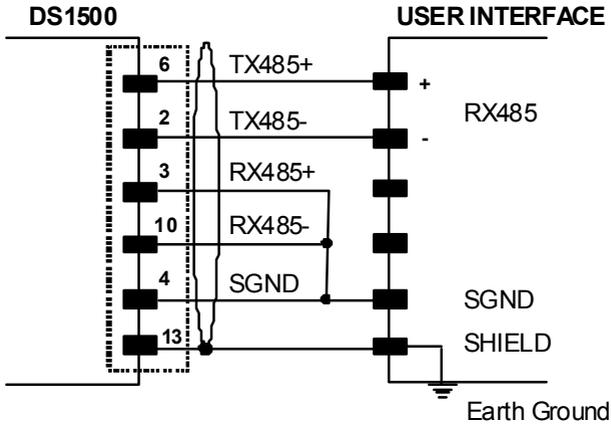
Figure 9 - RS485 Full-duplex Connections Using Only TX Signals
