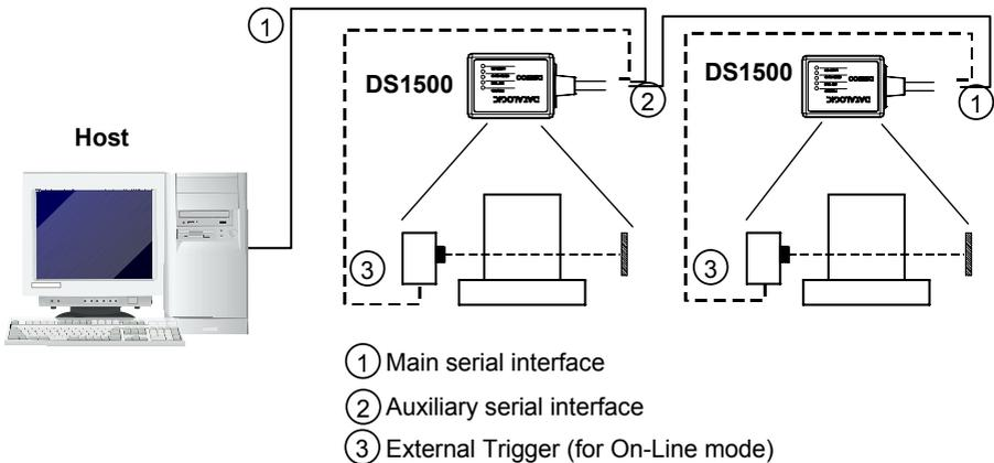
**Figure 21 – Pass-Through Layout**
