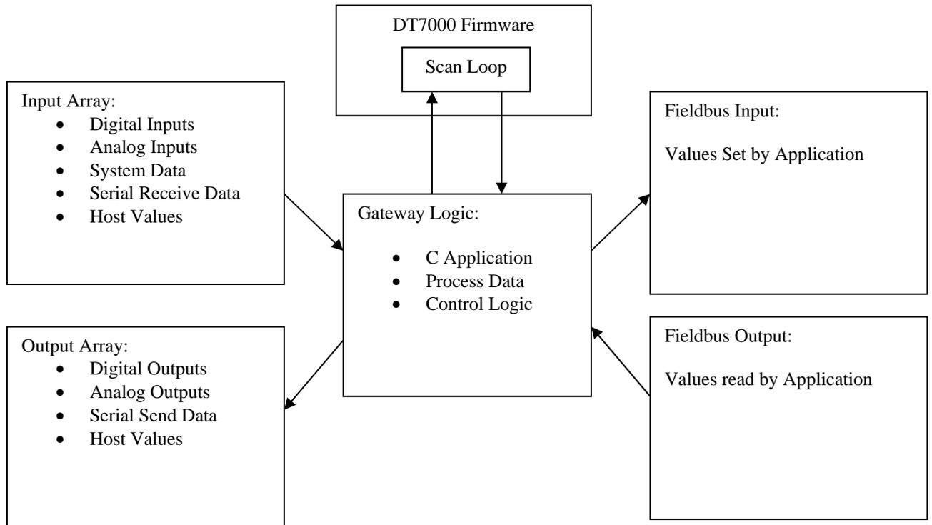
Figure 1 User Application Block diagram
