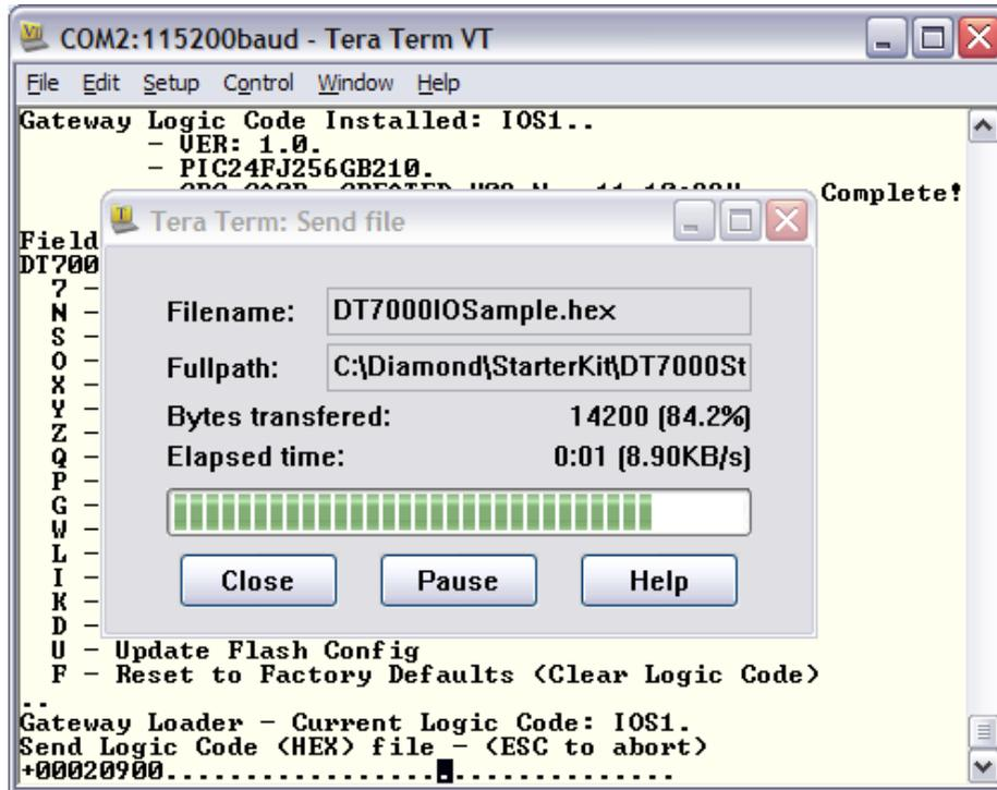
The DT7000 will display the address of application code as it is being downloaded to the DT7000.
